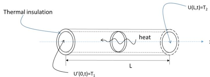
At  $t = 0$ , the temperature of interior nodes of the rod is zero and the boundary conditions are
